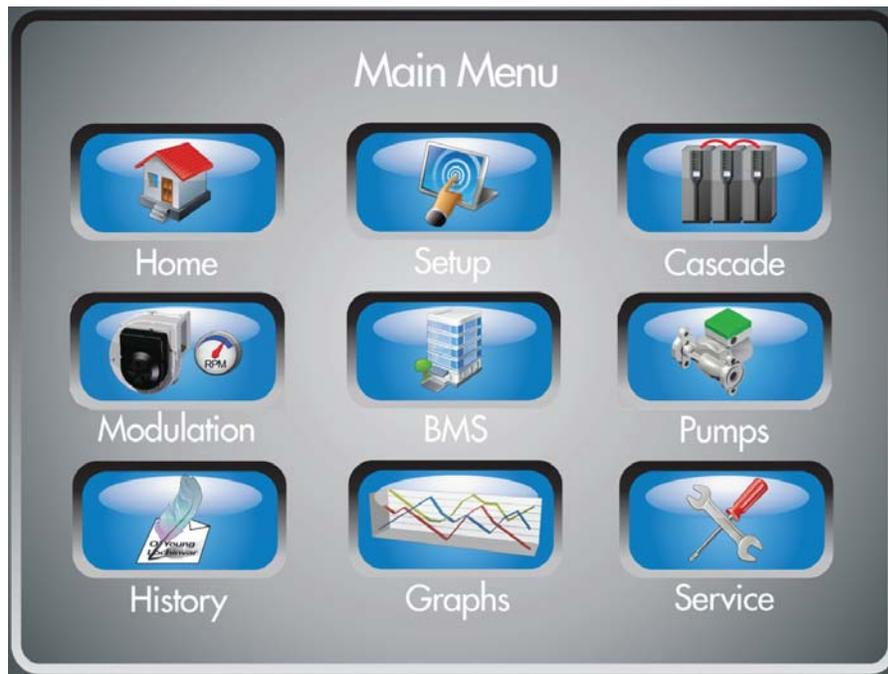
The Main Menu Screen allows navigation to nine (9) additional screens which are used to set temperatures, operating conditions, and monitor boiler operation. These screens are as follows:
