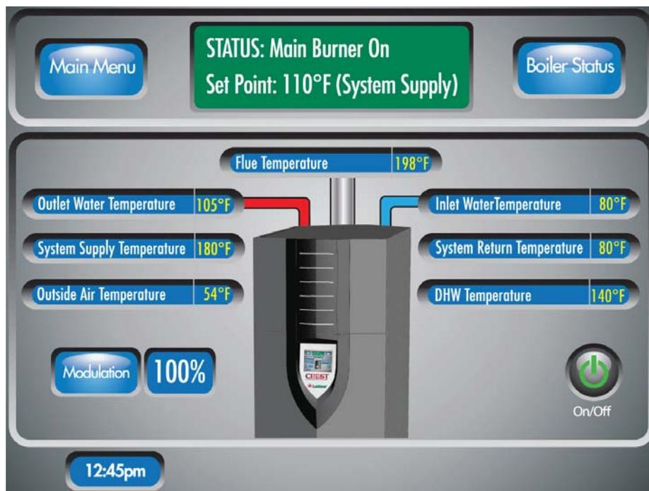
When the ON/OFF switch is turned to the ON position, the first screen visible on the LCD display will be the Home Screen. This screen displays the current status of the Crest boiler. The following items can be viewed or interacted with on the Status Screen:
